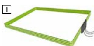
**J** If the Snail tape is fitted in a circle, repeat the actions as described in steps **G** and **H**, but now for the end of the Snail tape. Cut away any surplus length of Snail tape.
